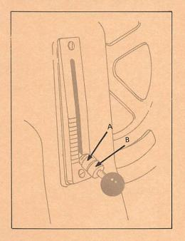
Adjust Stitch length by serrated nut (A) and tighten nut (B) against nut (A)
